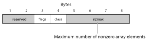
Figure 1-9, Array Flags Format for Sparse Arrays
